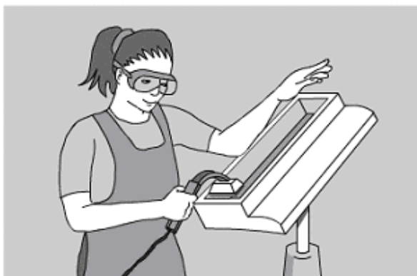
Example of a jig that corrects for faulty wrist posture
